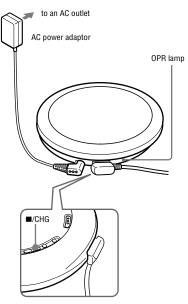
When the battery is completely charged, all indications on the display disappear and the OPR lamp goes off.
